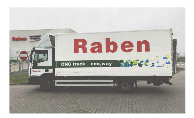
Their advantages include benefits for the environment: slightly lower emissions, and above all, almost no particulate matter and a reduction in noise by about 10 dB compared to diesel engines, which is important for deliveries in built-up areas.
